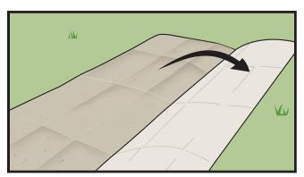
Fold top sheet open and pull back over anchored side.
