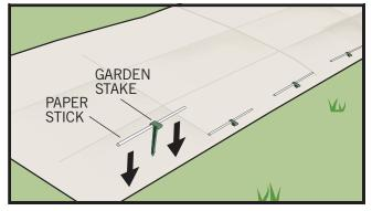
For best results, cut grass as low as possible before utilizing the Lazy Crazy Garden System. Lay system on the ground with TOP SHEET label facing up. Install 10 anchors along one side 3" from edge of sheet.
