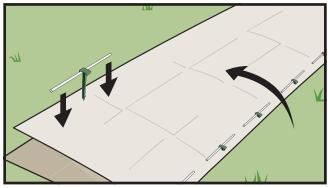
Fold top sheet over soil and seeds and anchor the remaining three sides. Install anchors 3" from each edge. Use 10 anchors per side and 2 per end of main unit.
